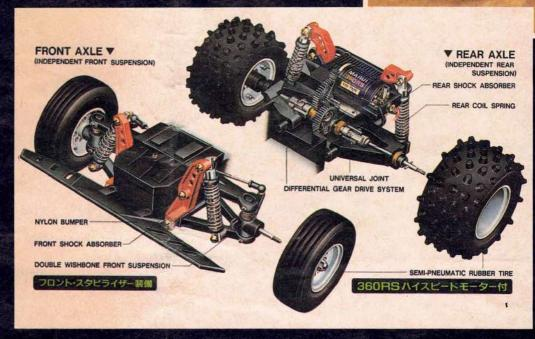
motor (550 type) through a metal pinion to plastic geared layshaft and plastic differential gear, outputting via substantial universal joints held in place by chunky set screws.
